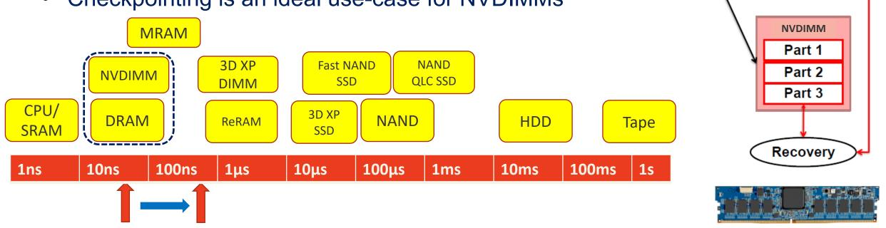
• NVDIMMs allow checkpointing to be done at DRAMs speeds (ns vs. μs)
